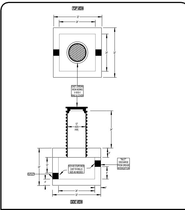
MFG. PER ASTM C478-5000# REINFORCED CONCRETE IN 28 DAYS
